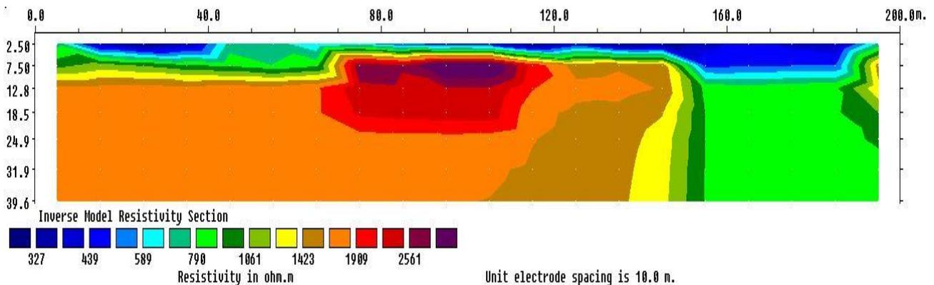
Figure 5: Inverse 2D Model Resistivity section along Profile 3
