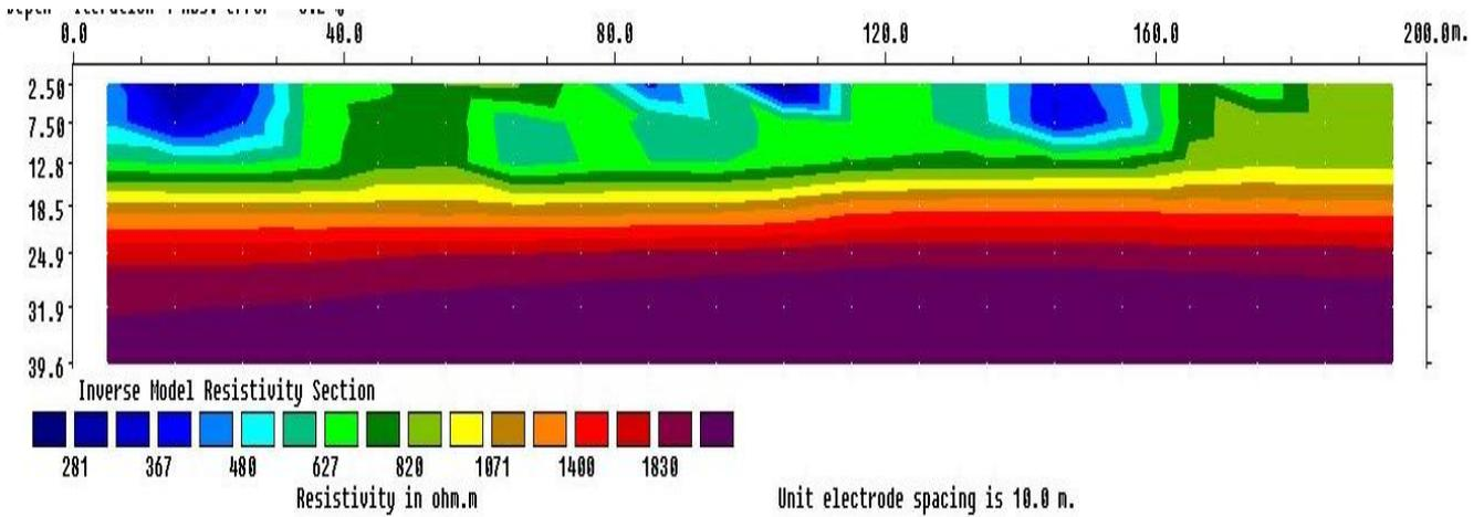
Figure 6: Inverse 2D Model Resistivity section along Profile 4
