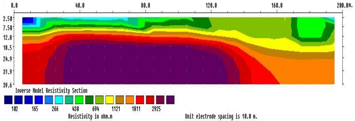
Figure 3: Inverse 2D Model Resistivity section along Profile 1
