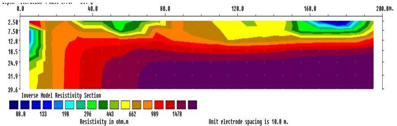
**Figure 12: Inverse 2D Model Resistivity section along Profile 10**
