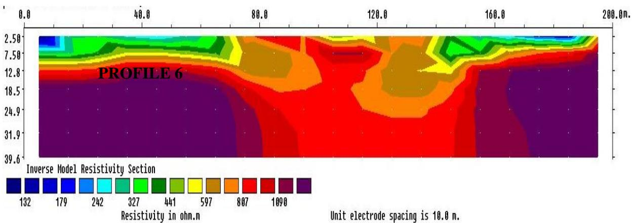
Figure 8: Inverse 2D Model Resistivity section along Profile 6
