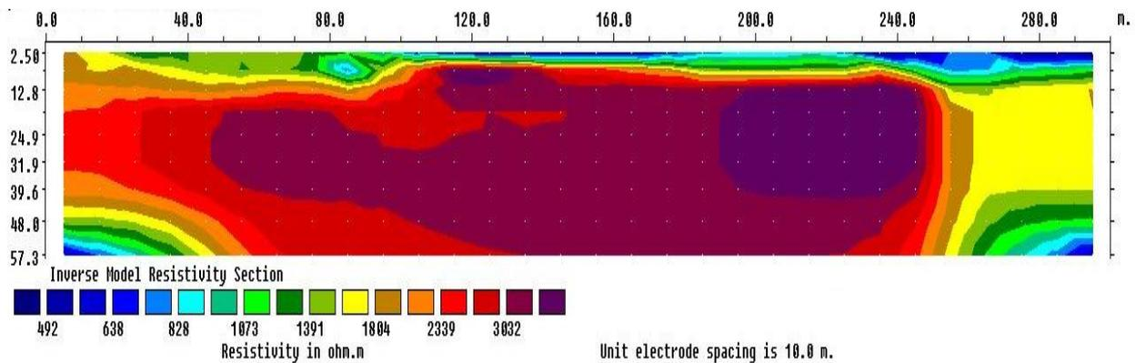
Figure 4: Inverse 2D Model Resistivity section along Profile 2
