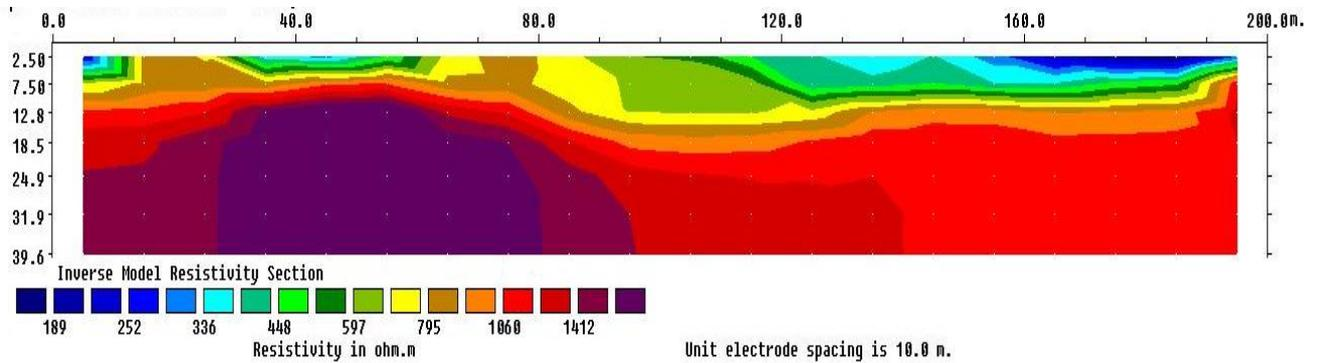
Figure 7: Inverse 2D Model Resistivity section along Profile 5
