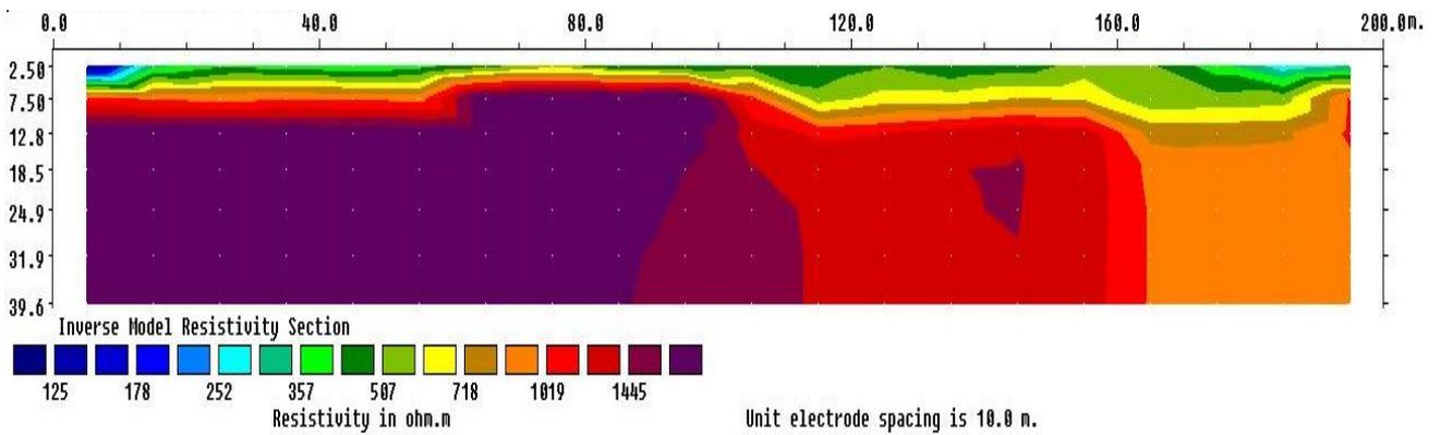
**Figure 10: Inverse 2D Model Resistivity section along Profile 8**
