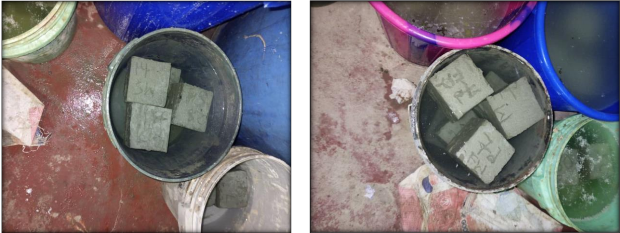
Figure 8: Curing of sample Concrete cubes.
