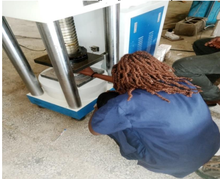
Figure 9: Testing the Compressive Strength of the Concrete Cubes
