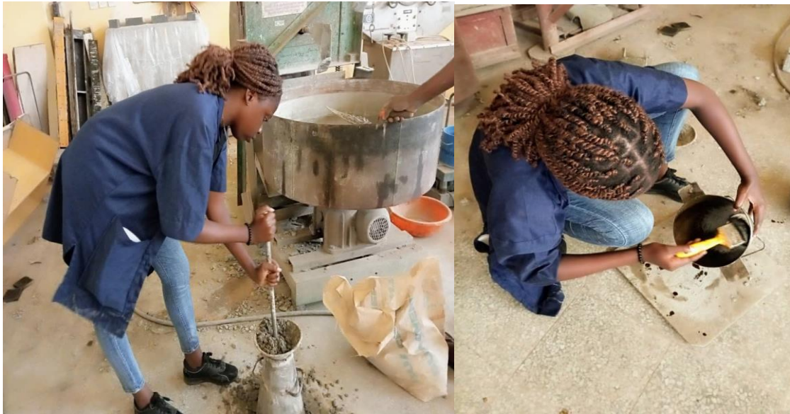
1.4 Figure 6: Slump Test on Concrete in Action
