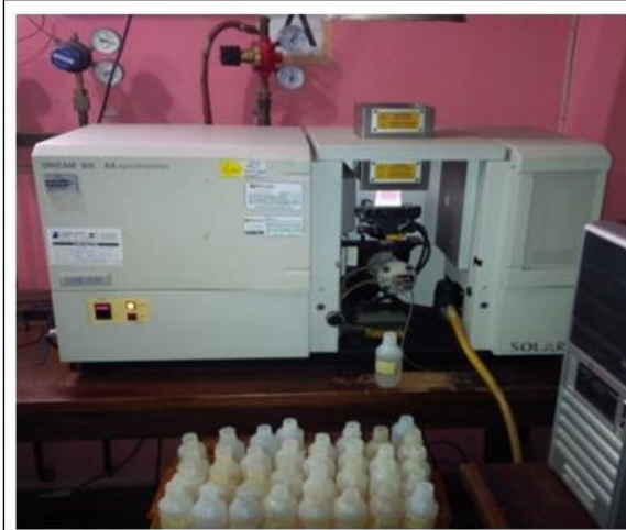
Figure 3: UNICAM 969 AA Spectrometer
