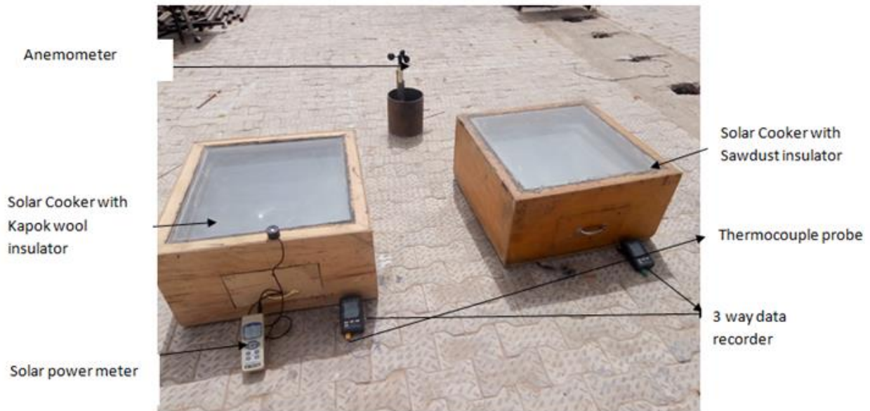
Plate 1: Experimental set up of the two similar solar box cookers
