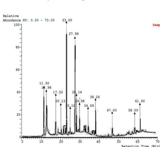
**Figure 5: GC-MS Analysis of Mango Biodiesel Produced**
