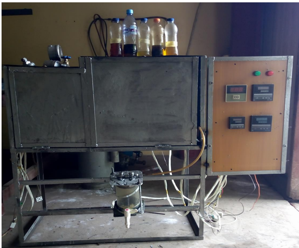
Figure 2: The Local waste plastics pyrolysis plant
