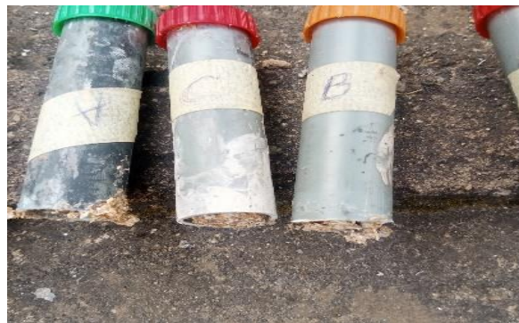
Figure 7: Briquette samples inside pipes (molds)
