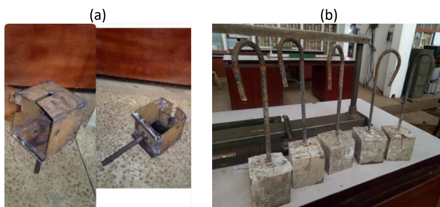
Figure 2: (a) Concrete bracket for holding concrete cubes (b) concrete cubes after testing showing cracks at interface between concrete and rebar
