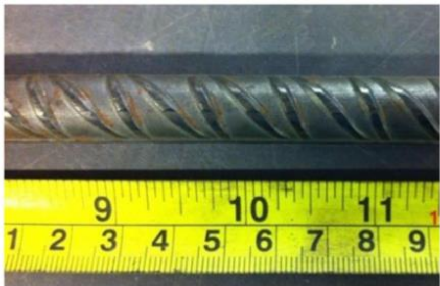
Figure 1: Picture of 12mm diameter steel reinforcing bar
