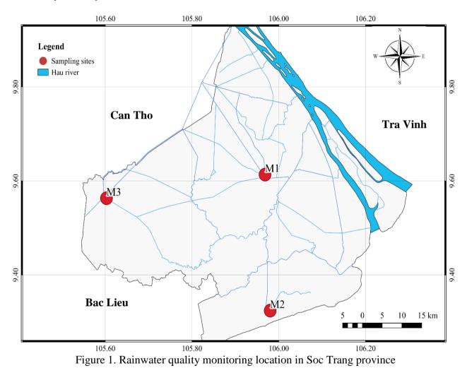
Water quality monitoring parameters include the pH, sulphate  $(SO_4^{2-})$ , nitrite  $(N-NO_2^{-})$ , nitrate  $(N-NO_3^{-})$ , ammonium  $(N-NH_4^{+})$ , sodium  $(Na^+)$ , calcium  $(Ca^{2+})$  and chloride  $(Cl^{-})$ . The pH parameters were measured in the field while the remaining parameters were analysed in the laboratory using standard methods [7].
