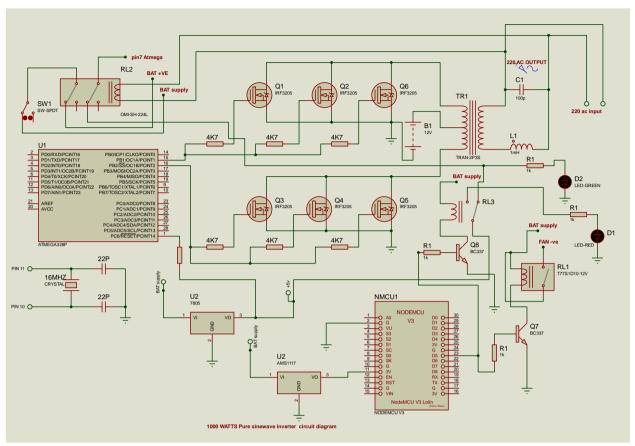
Fig 4: Circuit diagram of Wi-Fi controlled inverter simulated from Proteus
