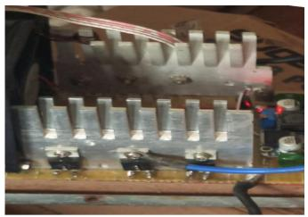
Fig 1: MOSFET placed on a heat sink
