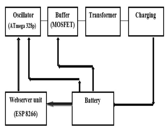
Fig 3: Block diagram of Wi-Fi controlled inverter
