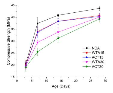
Figure 1: Compressive strength development for the various mixes
