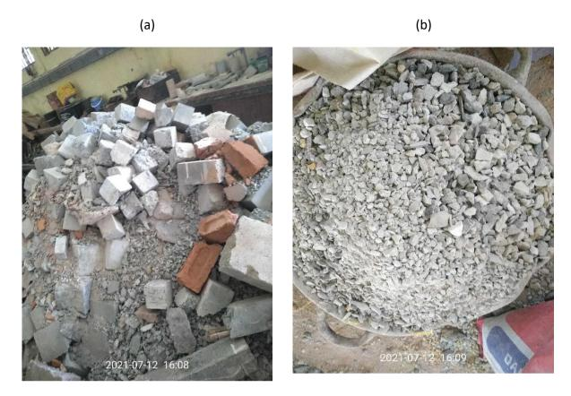
Plate 1: (a) Recycled concrete dumpsite (b) Extracted aggregates from the recycled concrete
