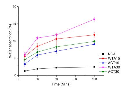
Figure 2: Percentage of water absorbed by the various concrete samples
