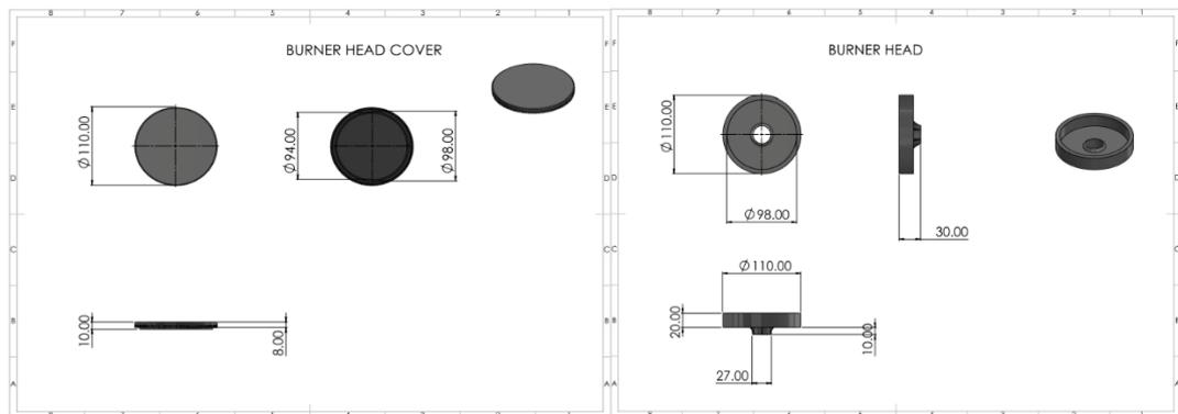
Fig 2. Burner Head Cover Drawings
