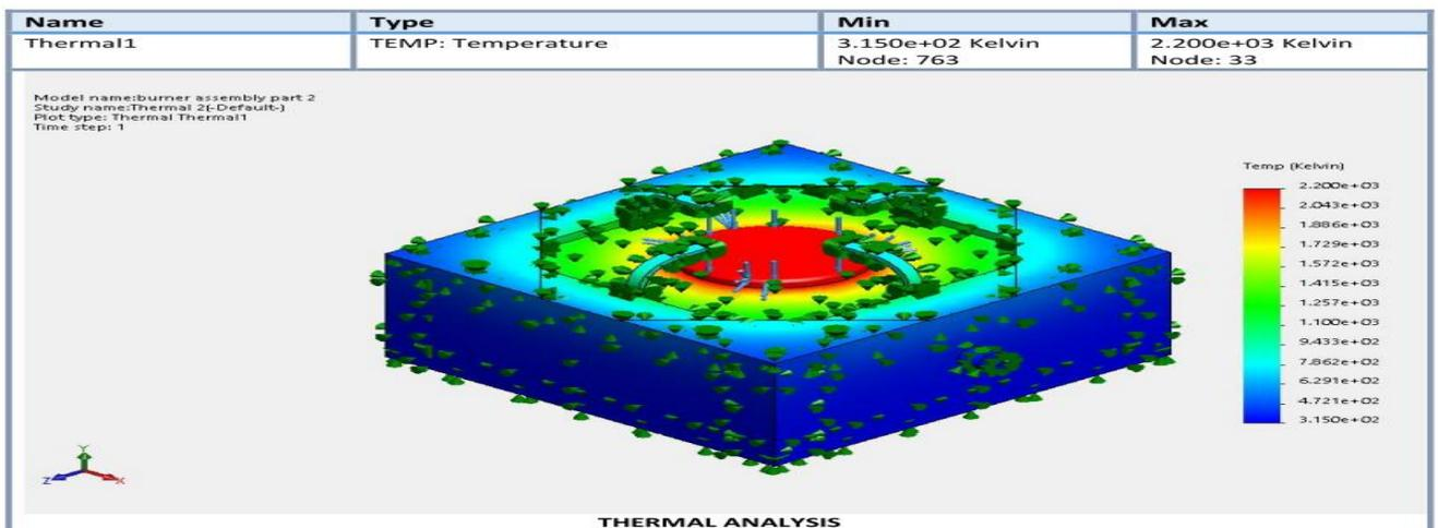
Figure 11. Thermal Analysis of Biogas Stove with Aluminum Burner
