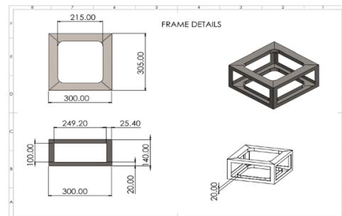
Fig 4 Biogas Stove Frame Drawing
