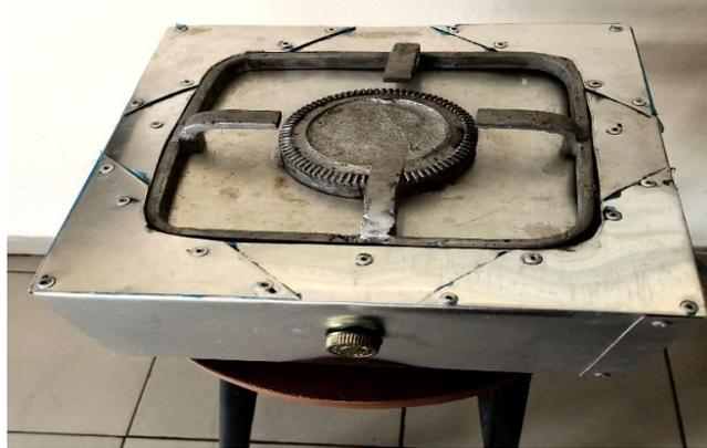
Fig 5: Actual Picture of the Fabricated Biogas Burner/Stove with Aluminum alloy Scraps
