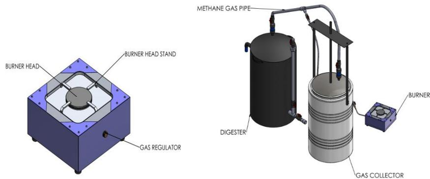
Fig. 6: Biogas Digester and Stove System Setup
