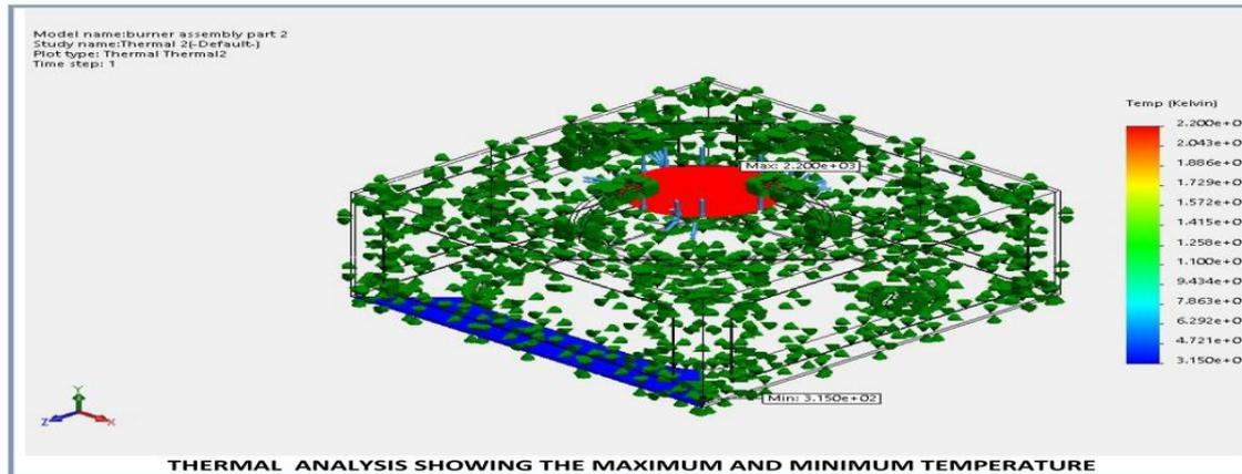
Figure 12. Thermal Analysis Showing the maximum and Minimum Temperature
