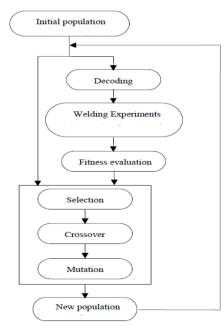
Figure 1: Optimization procedure using genetic algorithm.
