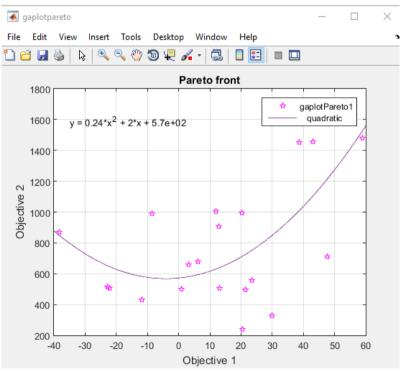
Figure 7: Pareto front plot showing objective function values
