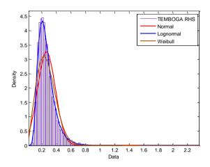
Figure 3: Probability Density Frequency of FoS of the gully wall RHS slope stability
