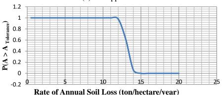
Figure 7: Graph of probability of rate of annual soil loss exceeding the tolerable or permissible rate against rate of annual soil loss for Ekhaguere gully using monthly rainfall data from CBN
