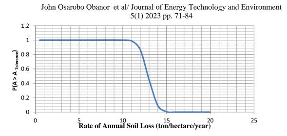
Figure 6: Graph of probability of rate of annual soil loss exceeding the tolerable or permissible rate against rate of annual soil loss for Ekhaguere gully using daily rainfall data from NIMET (1982 - 2011)
