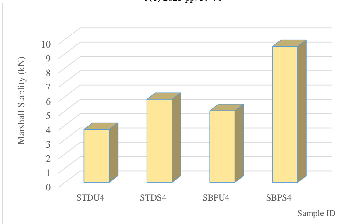
Figure 6: Marshall stability values for 4% filler
