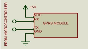
Figure 6: GPRS Module Unit
