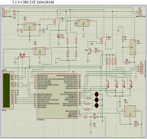
Figure 11: Circuit diagram
