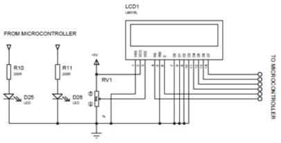
Figure 8: Display Circuit
