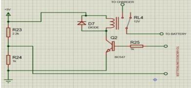
Figure 5: Charger Controller Unit
