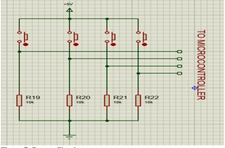
2.1.6 DESIGN OF THE KEYPAD (Button Circuit)
