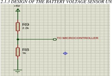
2.1.3 DESIGN OF THE BATTERY VOLTAGE SENSOR UNIT
