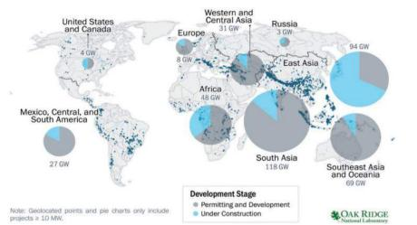
Fig. 4. Map of hydropower project development by region and development stage, end of 2019 [49]
