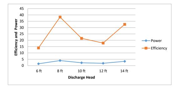
Figure 8: Plot of power and efficiency at 4.0 ft supply head against varying discharge head
