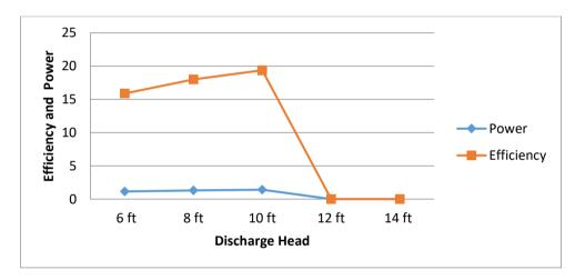
Figure 7: Plot of power and efficiency at 2.8 ft supply head against varying discharge head
