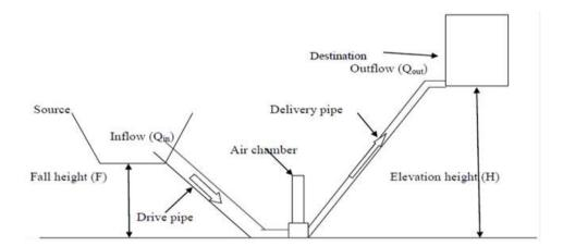
Figure 1. Schematics of the working actions of a hydraulic ram pump [13]
