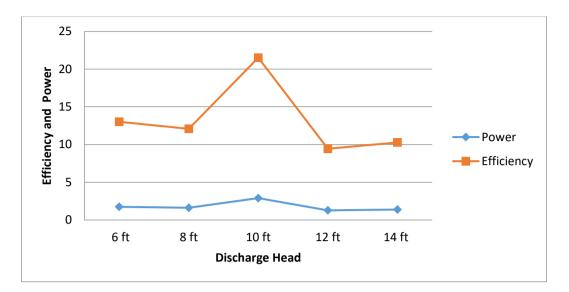
Figure 9: Plot of power and efficiency at 5.2 ft supply head against varying discharge head
