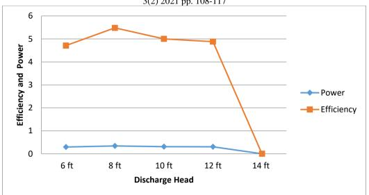
Figure 6: Plot of power and efficiency at 2.4 ft supply head against varying discharge head
