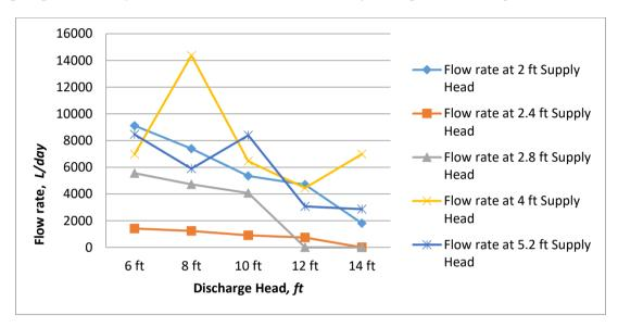
Figure 4: Plot of flow rate of varying supply head against varying discharge head
