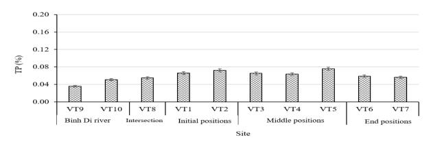
Figure 6. Total phosphorus concentrations in sediments in dry season
