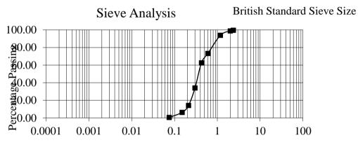
Figure 1: Sieve analysis of fine aggregate
