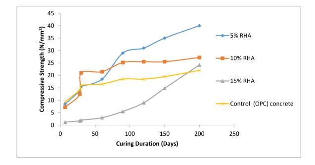
Figure 2: Compressive strength and curing period at 0%-15% RHA concrete
