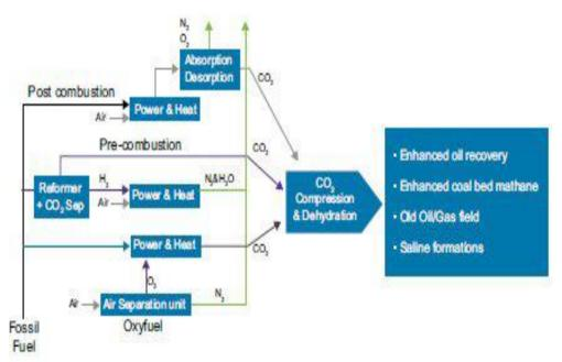
Figure 3- Schematic overview of the three processes of CO<sub>2</sub> capture technologies [17].
