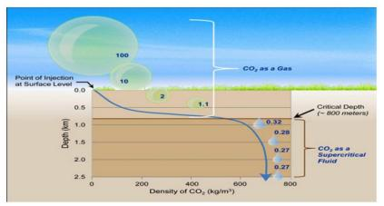
Figure 9. Changes in  $CO_2$  phases at the point of injection. (Source: NETL, Department of Energy (DOE) US).
