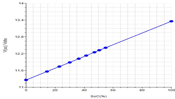
**Figure 3:** Graph of SoC against V(oc) for Luminous Battery
