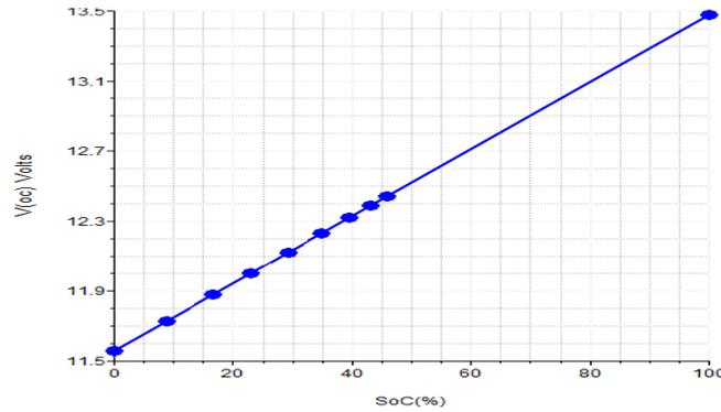
**Figure 4:** Graph of SoC against V(oc) for Mercury Battery
