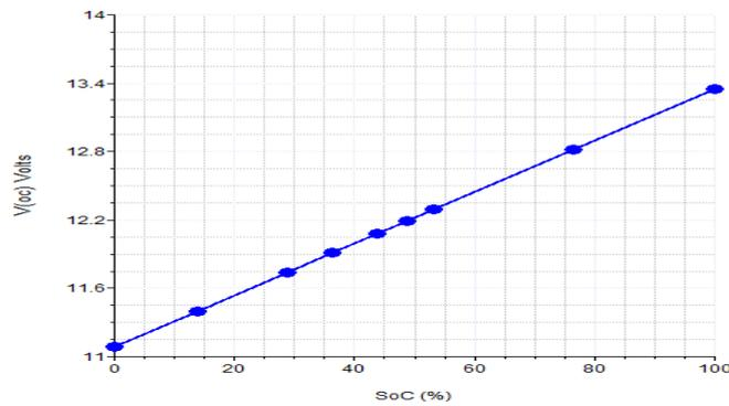
**Figure 2:** Graph of SoC against V(oc) for Safepower Battery
