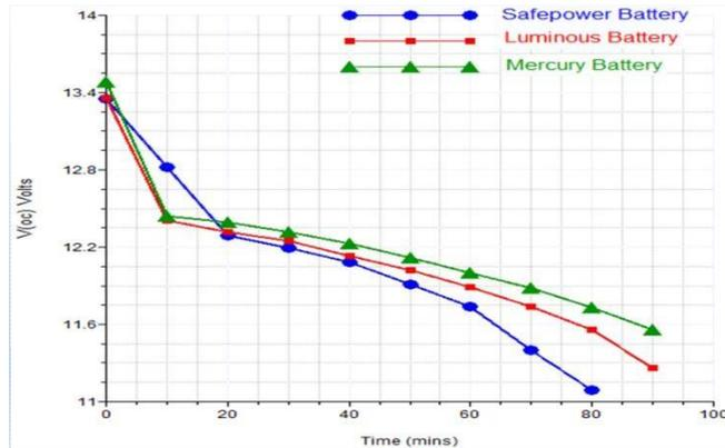
**Figure 1:** A graph of V(oc) against time for the three batteries
