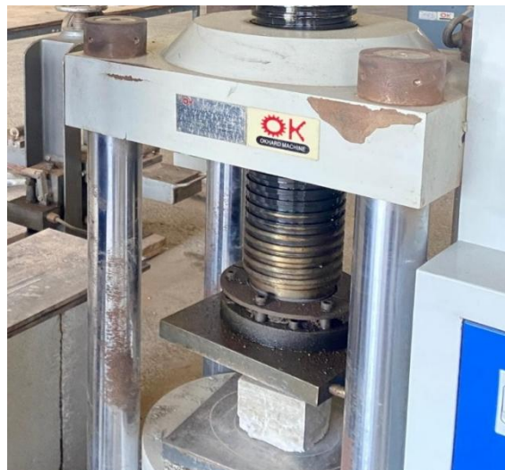
Figure 6: Compression Test on Cubes in the Laboratory.
