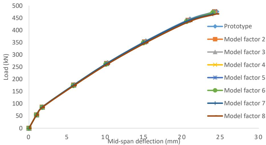
**Figure 7 Load-deflection curve for the prototype and the predicted prototype beams**
