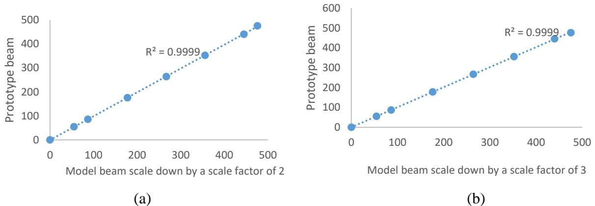
**Figure 8: (a) Prototype vs predicted prototype beam by a scale factor of 2; (b) Prototype vs predicted prototype beam by a scale factor of 3**
