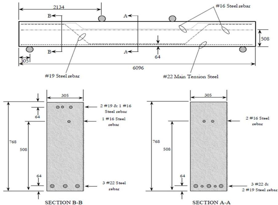
Figure 1: Typical steel reinforcement locations [21]
