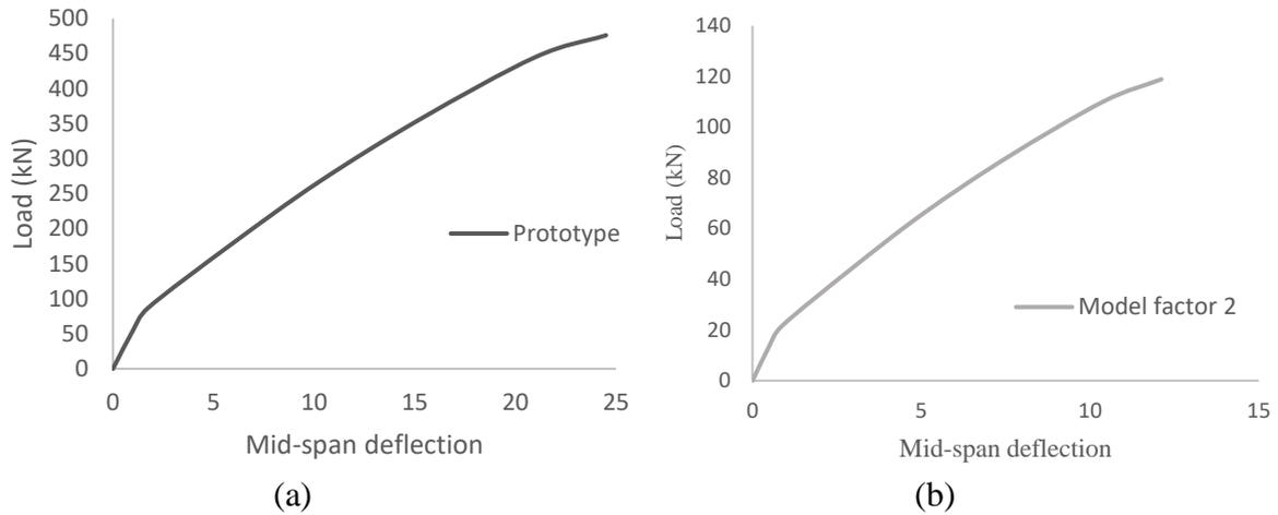
**Figure 3: Load-deflection curve (a) the Prototype beam [21]; (b) model beam scale down by a scale factor of 2**
