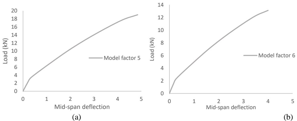
**Figure 5: Load-Deflection Curve. (a) model beam scales down by a scale factor of 5; (b) model beam scale down by a scale factor of 6**
