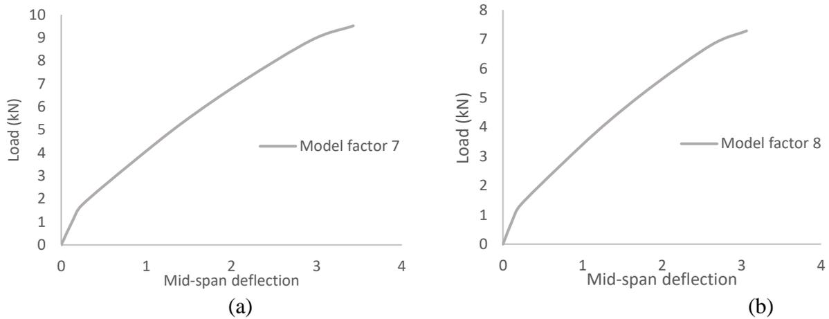
**Figure 6: Load-Deflection Curve. (a) model beam scale down by a scale factor of 7; (b) model beam scale down by a scale factor of 8.**
