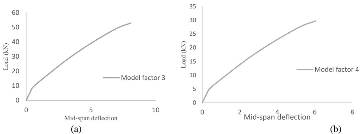
**Figure 4: Load-Deflection Curve. (a) model beam scales down by a scale factor of 3; (b) model beam scale down by a scale factor of 4.**
