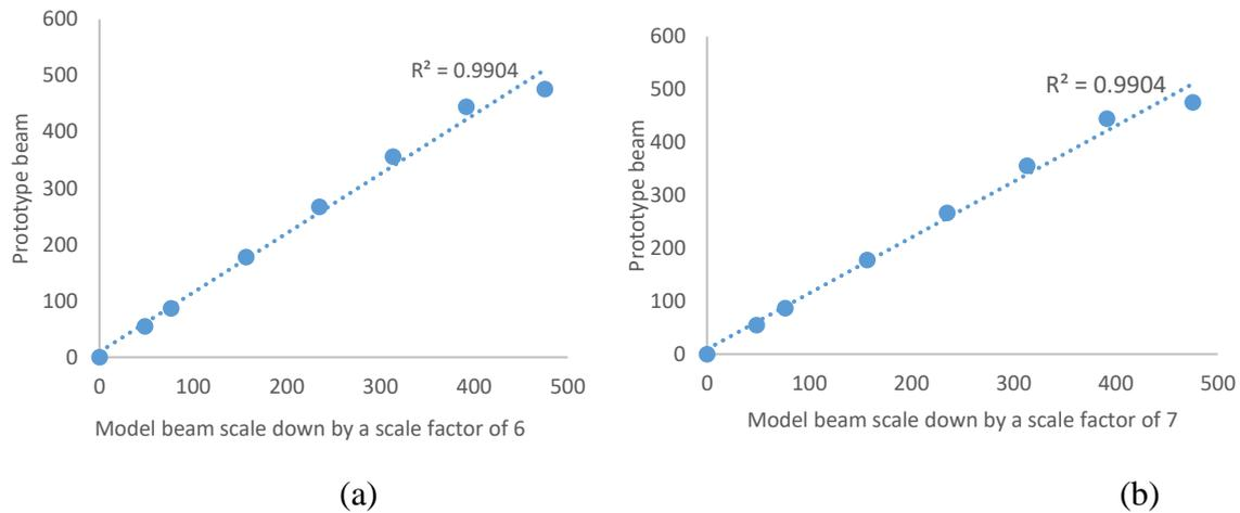
**Figure 10: (a) Prototype vs predicted prototype beam by a scale factor of 6; (b) Prototype vs predicted prototype beam by a scale factor of 7**
