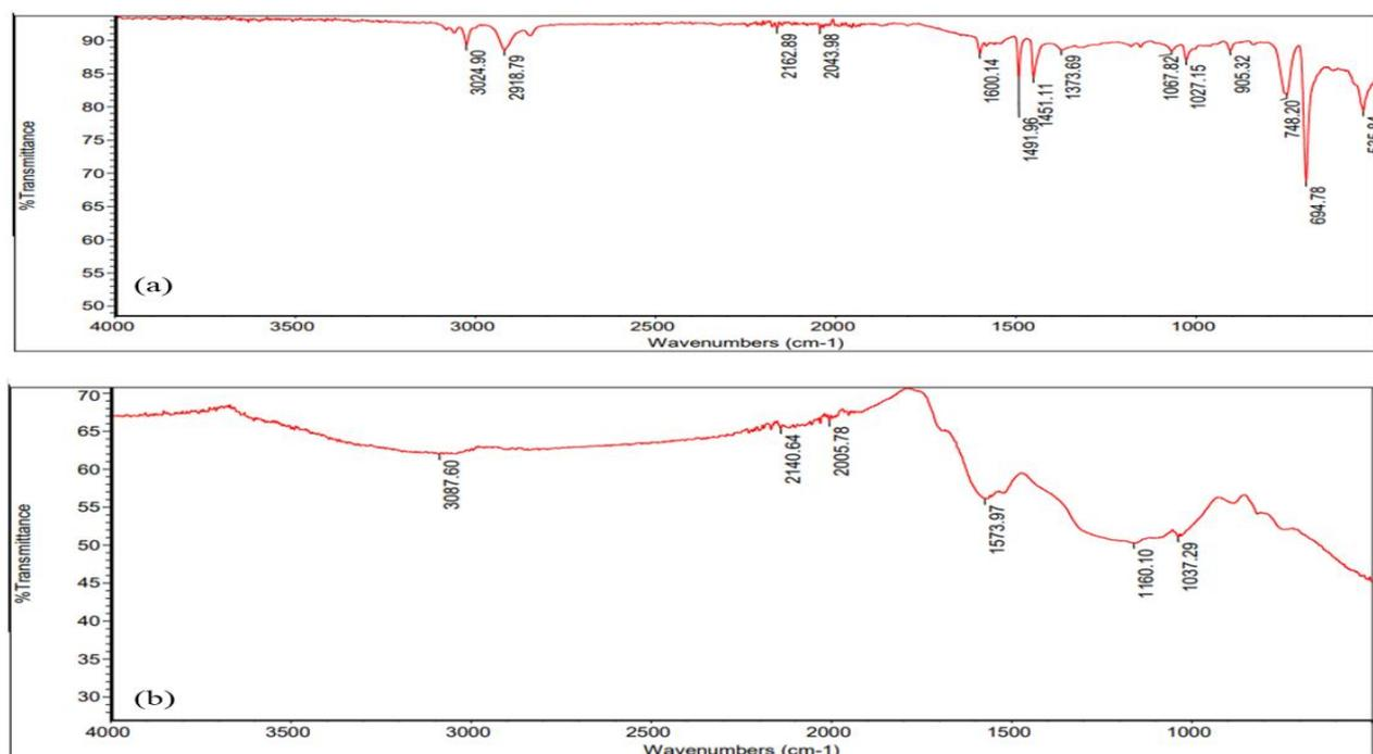
**Fig.1:** FT-IR spectra for (a) coconut coir activated carbon (b) keratin-based coconut coir activated carbon composite.
