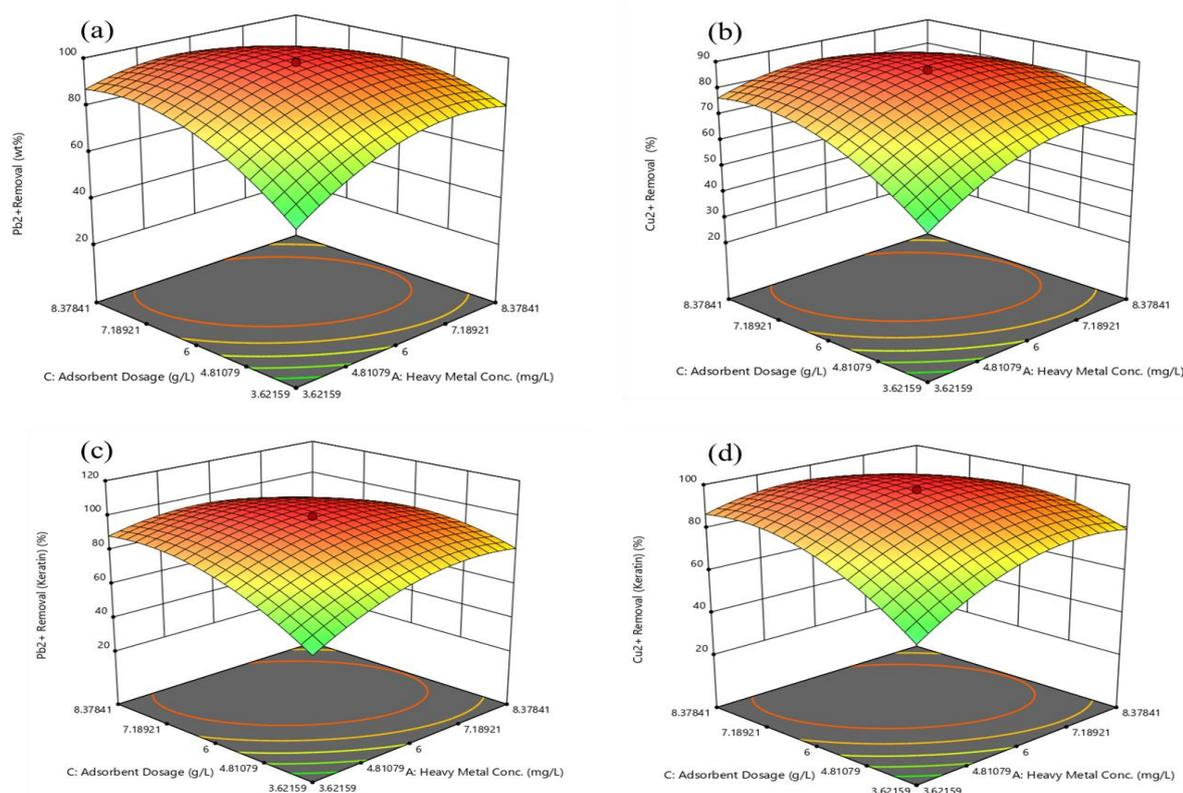
**Fig. 4:** 3D Response surface of effects of adsorbent dosage on the concentration of (a) Pb<sup>2+</sup> and (b) Cu<sup>2+</sup> removal using coconut coir activated carbon (c) Pb<sup>2+</sup> and (d) Cu<sup>2+</sup> removal using keratin-based coconut coir activated carbon composite.
