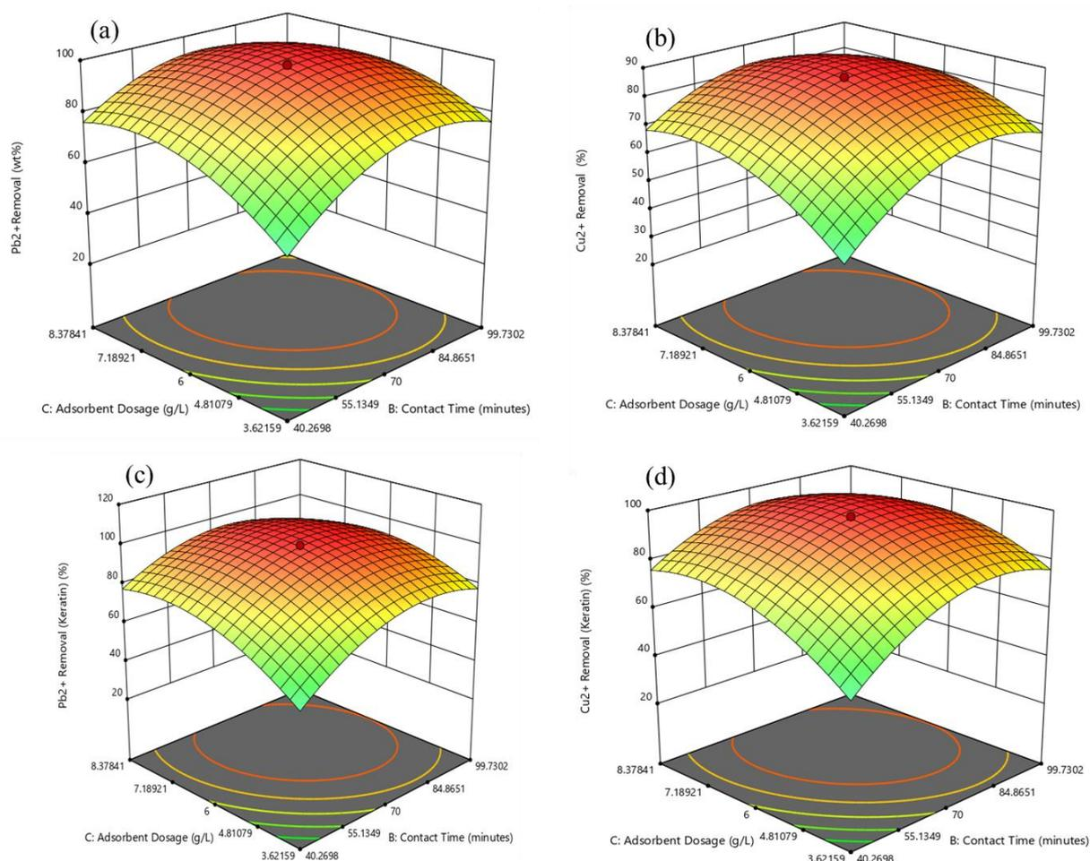
**Fig. 5:** 3D plots of the effect of contact time in relation to adsorbent dosage for (a) Pb<sup>2+</sup> (b) Cu<sup>2+</sup> Coconut coir activated carbon and (c) Pb<sup>2+</sup> (d) Cu<sup>2+</sup> keratin based activated carbon composite.
