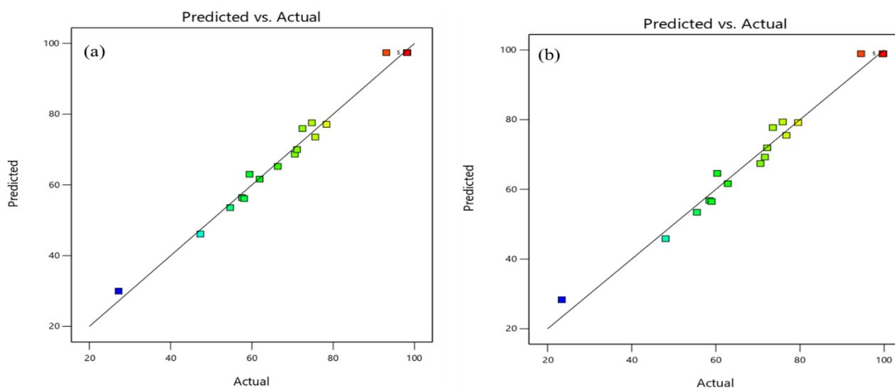
**Fig. 6: Parity plot of predicted against actual Pb<sup>2+</sup> ions removal for (a) coconut coir activated carbon and (b) keratin-based coconut coir activated carbon composite.**
