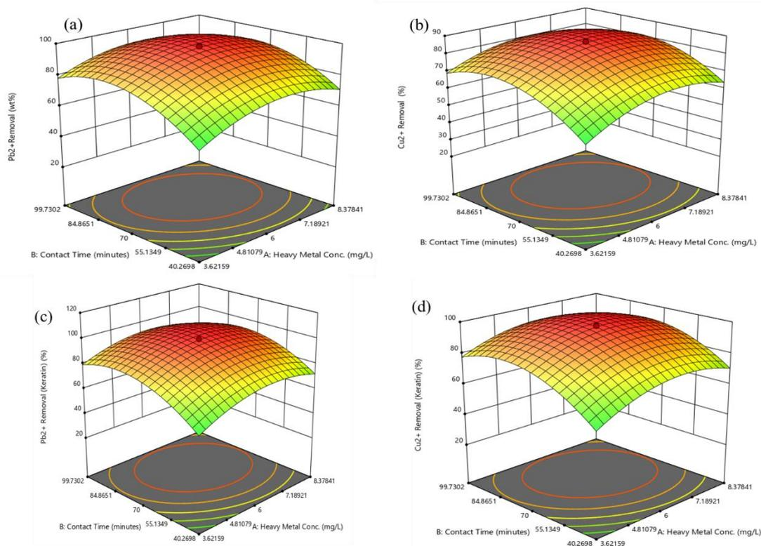
**Fig. 3:** 3D Response surface of effects of contact time on the concentration of (a) Pb<sup>2+</sup> (b) Cu<sup>2+</sup> removal using coconut coir activated carbon (c) Pb<sup>2+</sup> and (d) Cu<sup>2+</sup> removal using keratin-based activated carbon composite.
