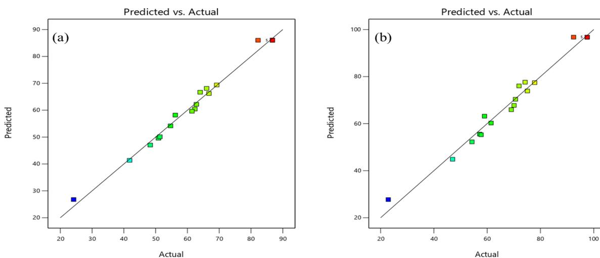
**Fig. 7: Parity plot of predicted against actual Cu<sup>2+</sup> ions concentrations for (a) activated carbon (b) keratin-based activated carbon composite.**
