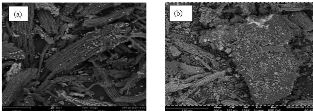
**Fig. 2: Scanning Electron Micrograph (a) activated carbon and (b) keratin-based activated carbon composite.**
