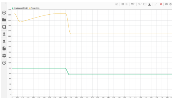
Figure 10a: Output Power P&O optimized system
