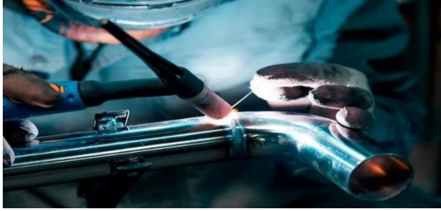
Figure 1: A. Tungsten Inert Gas Welding (fractory.com)
