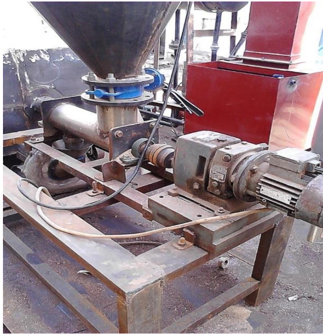
Figure 4: Fabricated Hopper-Screw Conveyor System
