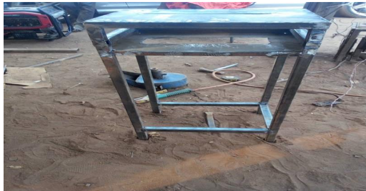
Figure 7: Construction Stage of the Paper Shredder
