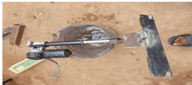
Figure 4: Linear Actuator with an Attached Die to the Notch
