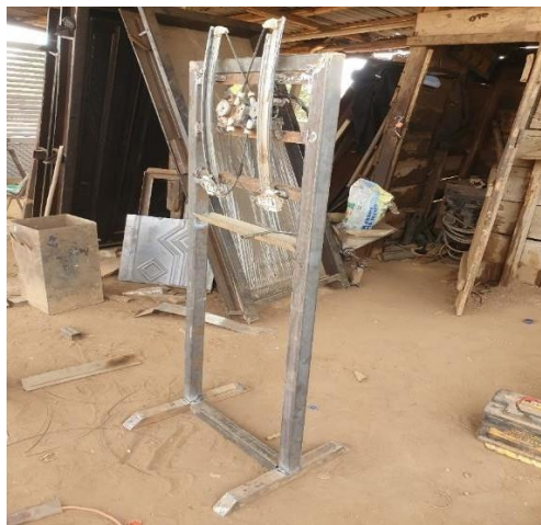
Figure 7: Actuator Assembling on the Automated Metal Sheet Bending Machine
