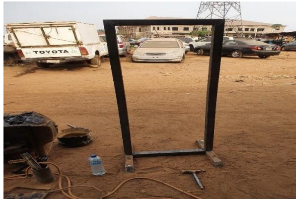
Figure 6: Metallic Frame of the Automated Metal Bending Machine
