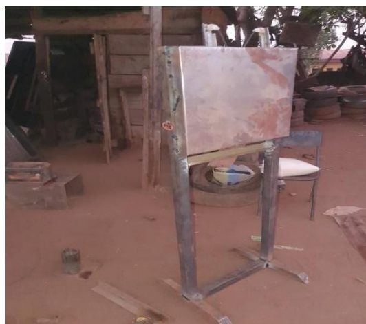
Figure 8: Assembling of the Automated Metal Sheet Bending Machine
