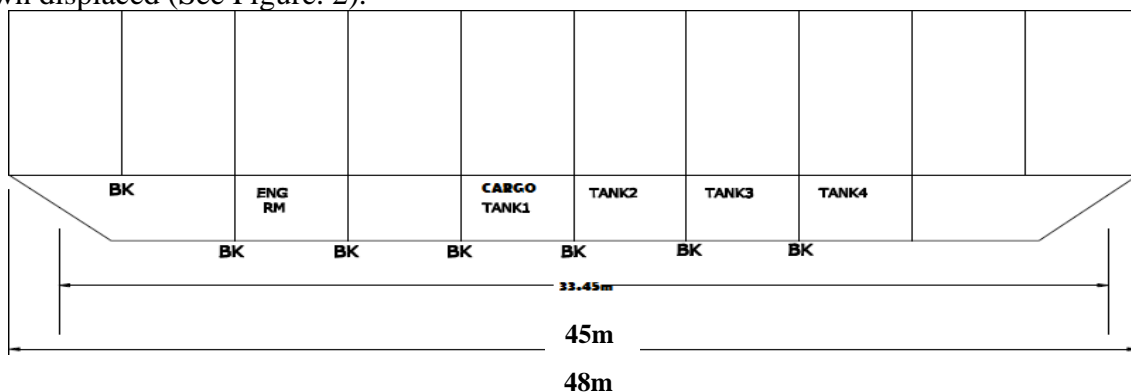
Figure 2. Arrangement of the Barge
