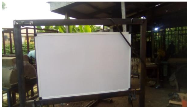
Figure 6 - Board Mounted on the Frame
