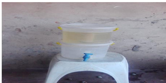
Fig 4: The set up for the filtration process
