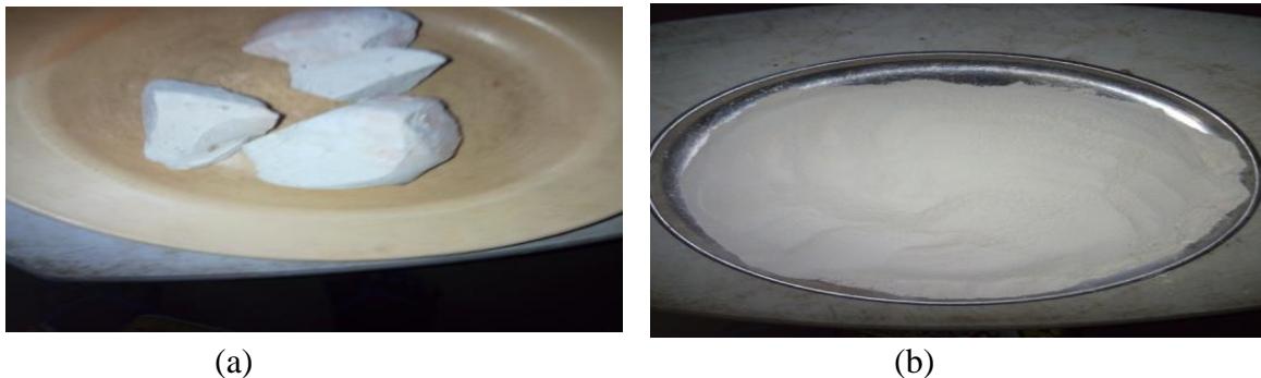
Fig 1: Sample of unprocessed (a) and grounded (b) kaolin
