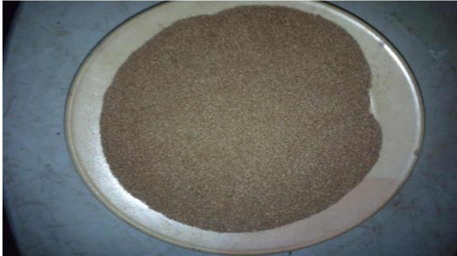
Fig 2: Sample of hardwood (sawdust) used as a pore forming agent
