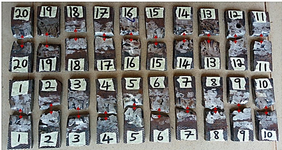
Figure 2: Test samples that have undergone tensile test from instron tensile test machine
