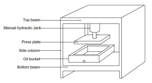
Figure 1. The manual hydraulic oil expeller
