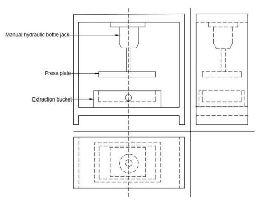
Figure 3 First angle orthographic projection of the press showing component parts
