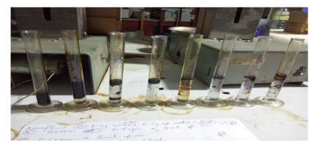
Figure 2. Recovery of Oil after flooding
