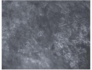
Plate 3c: Optical Micrograph of Austempered 0.3%C Steel at 320°C Immersed in Sea Water 45 Days - (200X)
