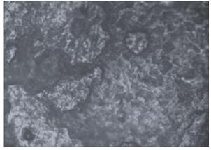
Plate 4b: Optical Micrograph of Austempered 0.3%C Steel at 300°C Immersed in Sea Water for 60 Days - (200X)
