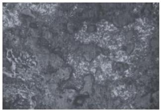
Plat 3a: Optical Micrograph of Control Sample of 0.3%C Steel Immersed in Sea Water 45 Days - (200X)
