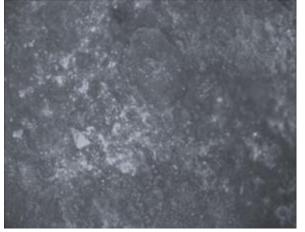
Plat 5a: Optical Micrograph of Control Sample of 0.3%C Steel Immersed in Sea Water 75 Days - (200X)
