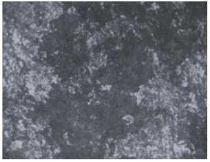
Plate 1d: Optical Micrograph of Austempered 0.3%C Steel at 340°C Immersed in Sea Water for 15 Days - (200X)
